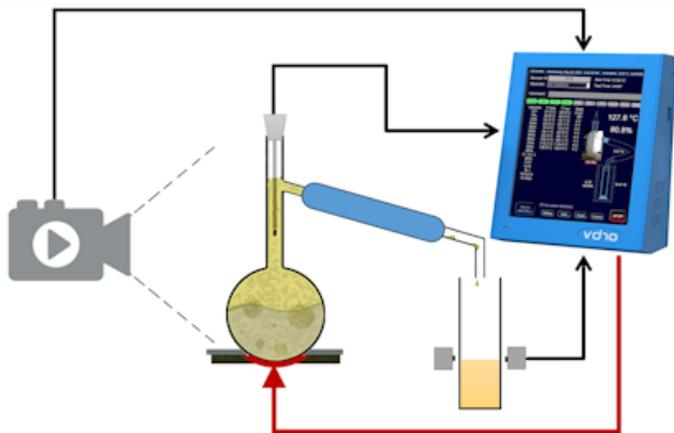
**The entire test procedure is fully automated:** position of the flask, its heating, condenser and receiver temperatures regulation, measuring vapor temperatures and volume, detecting IBP and FBP, rate control, perform barometric correction and recording all data. At test completion, the heater is automatically lowered and cooled down quickly. Results are displayed, saved, printed, sent to LIMS or USB.
